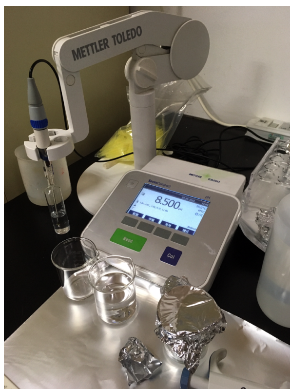
Adjusting pH of AAs samples before derivatization and injection in the HPLC.
